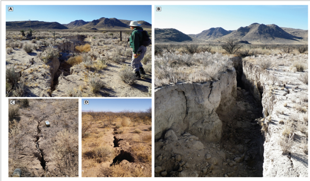
Figure 4. Field photos of newly opened earth fissures. A) A large open section of fissure C from figure 3, note fence stretched across open fissure. B) Deep, steep-sided section of the same fissure. C-D) Narrow surface cracks and aligned potholes representative of portions of earth fissures that have not yet opened completely. A subsurface void likely underlies these features and the overlying soil may one day collapse into it.
