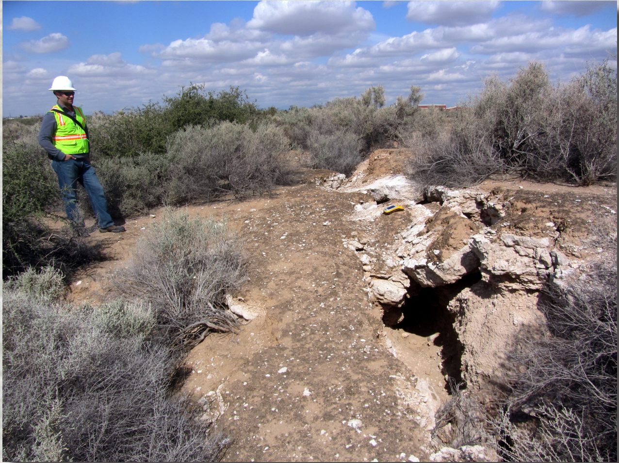
Strongly cemented carbonate beds drape across an earth fissure near Luke Air Force Base.
