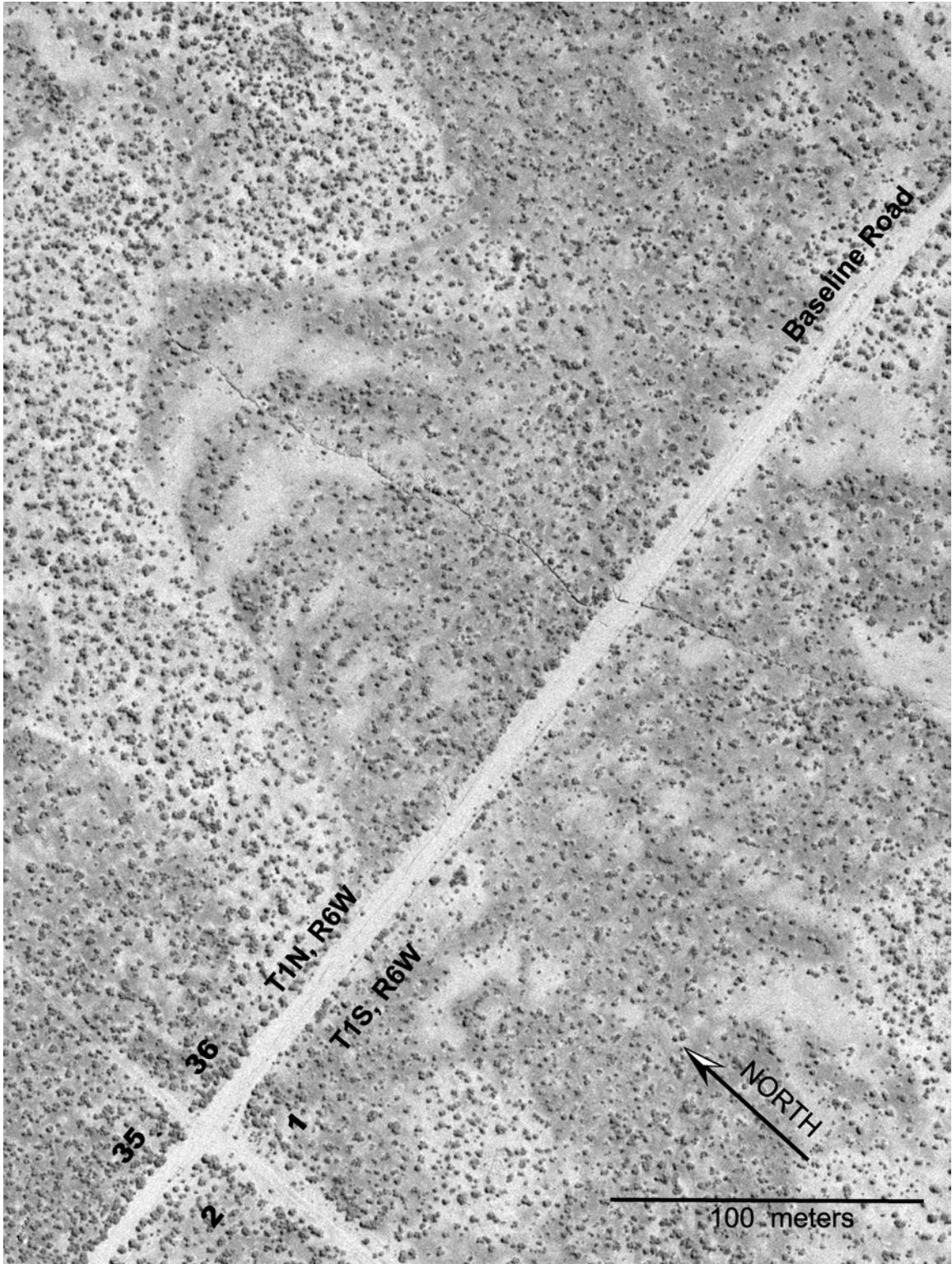
Figure 4. Detailed aerial view of new earth fissure.
