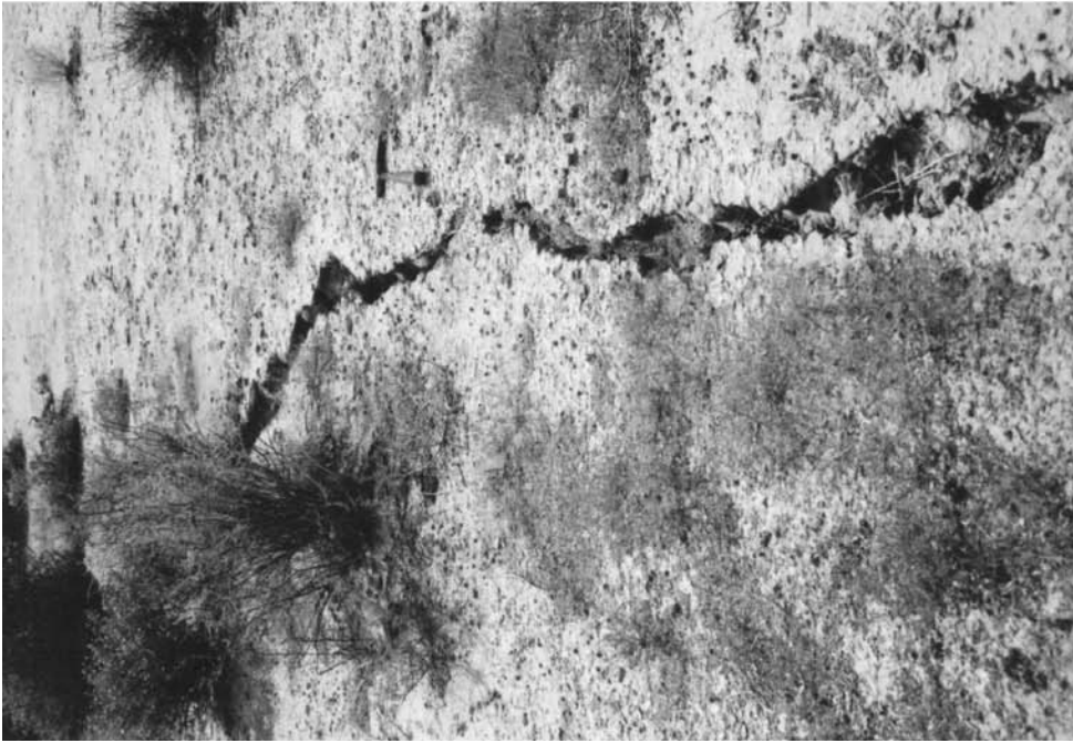
Figure 12. New desiccation crack, with vertical sides, sharp angles, and lack of vegetation. Rock hammer for scale.
