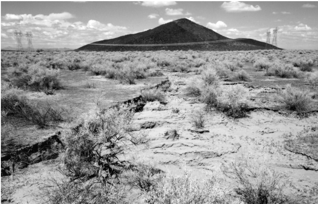
Figure 6. Section of earth fissure north of Baseline Road, showing erosion on uphill (east) side. Fissure is 12-18 inches wide, 1-6 feet deep in this section.
